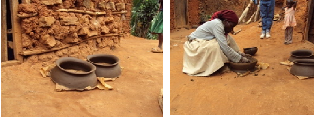
Plate 3: Pot making a) the top half of the pot and b) the bottom half of pots (the top is turned upside down)
